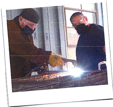
Left: Welders Owen Hatridge and Jonathan Ramirez use a plasma torch to cut metal to size.
